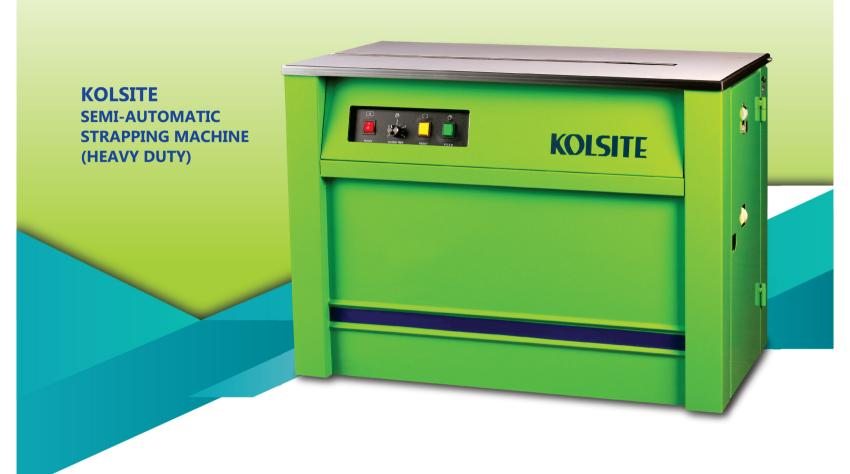
KOLSITE Semi-Automatic strapping machine designed to tension, seal and cut 6-15mm PP strapping around carton boxes. Simply load the strapping onto the machine and feed it through the mechanism Place the carton on top of the deck and feed the strap into the strap guide to activate the strapping process. The machine will automatically tension, seal and cut the strapping, giving a perfect strap every time.
